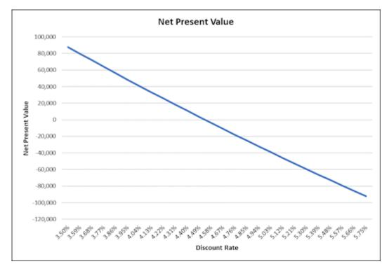
Per the graph above, the fixed rate is approximately 4.58% (NPV is approximately zero at that point).
